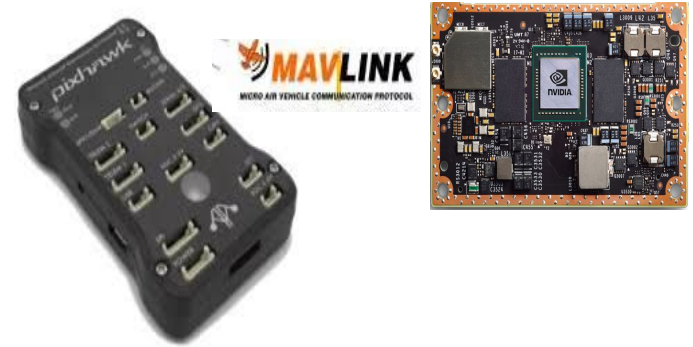
MAVROS link between Jetson and Pixhawk Controller
