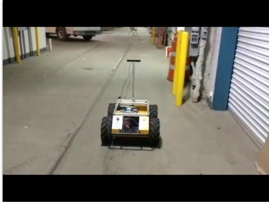
SLAM system test: from ORB SLAM2 to Intel Tracking Camera
