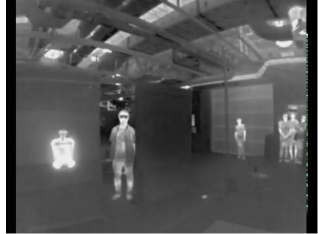
Fire source simulation/modeling: Using message bag filled with water as fire source.
