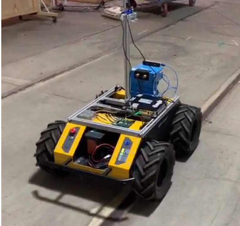
Current Husky with LIDAR, ZOTAC and PCB
