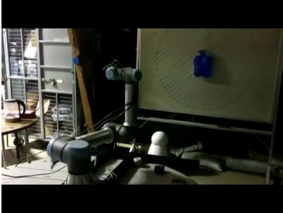
UR5e arm moving towards fire location using visual feedback
