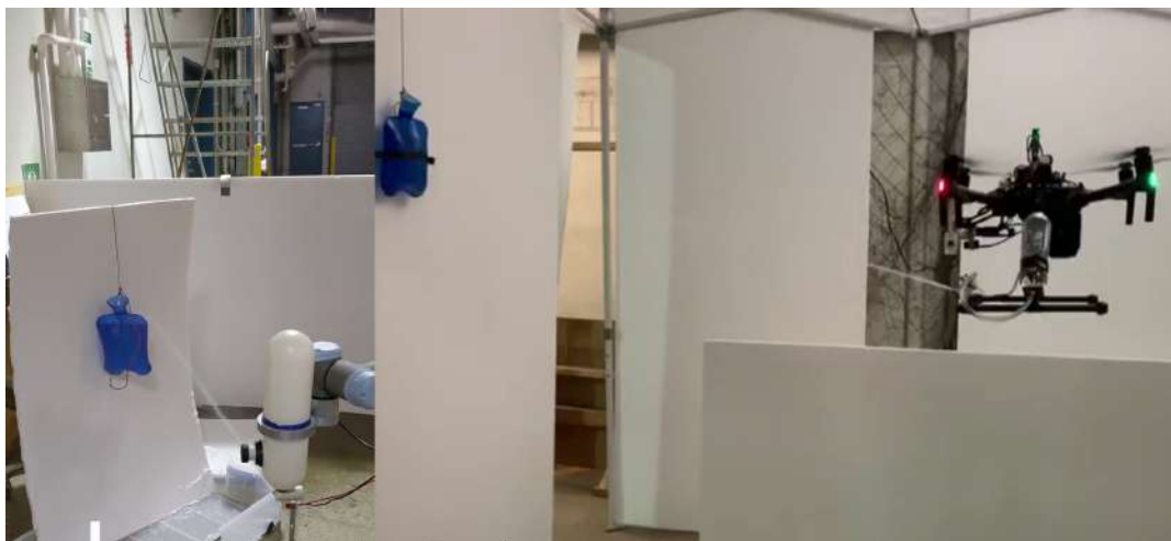
Figure 18: AGV water deployment (left) and UAV water deployment (right)
